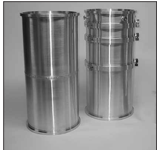
Modular vacuum chambers with ISO-320k flanges and lengths of 100, 200, 400 & 800 mm. Inside diameter is 362 mm.
