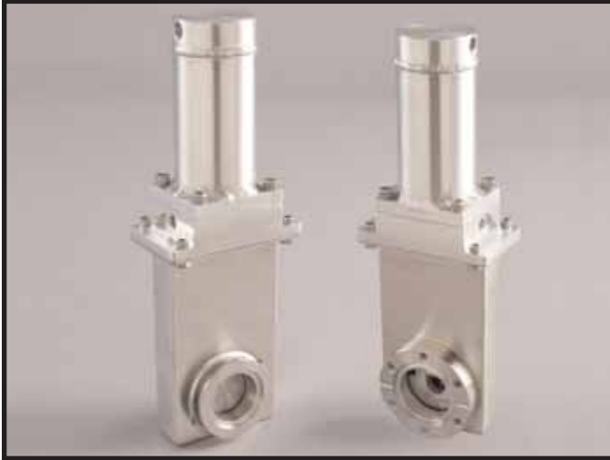
Valve on the left has NW-40 flange. Valve on the right has special 2.75 In. Conflat® flange. Standard practice is for bolt circle to straddle center line.
