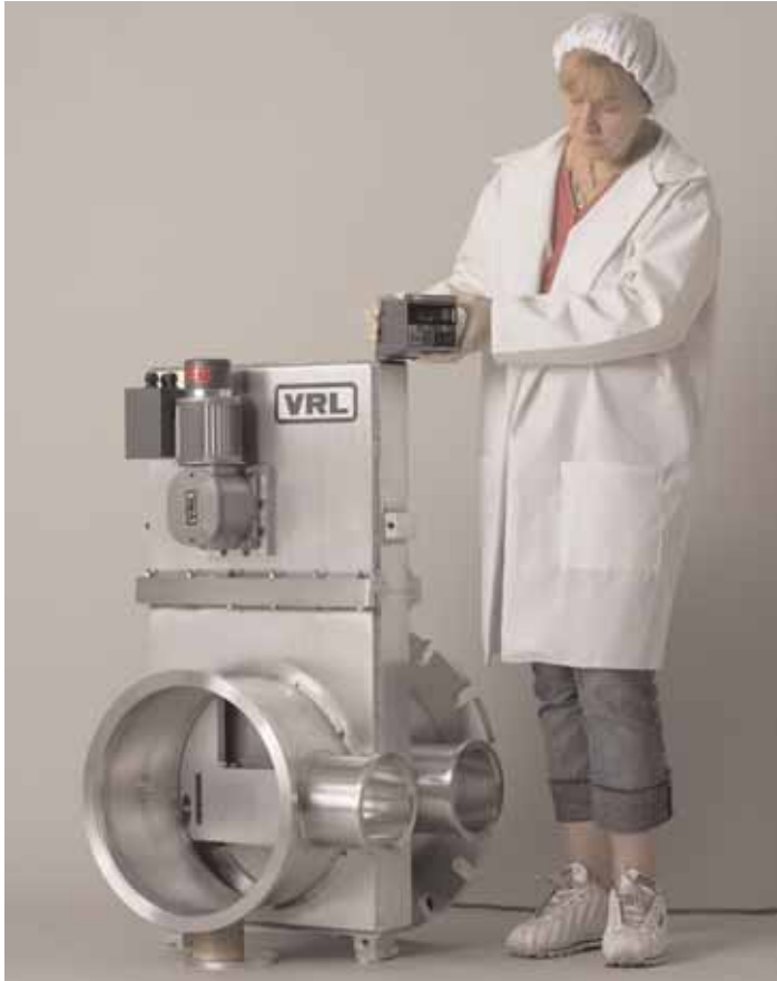
Throttle valve with ISO-400 flange on one side and 16 inch ANSI flange on the other. An ISO-100 roughing port is located on both sides of the gate.
