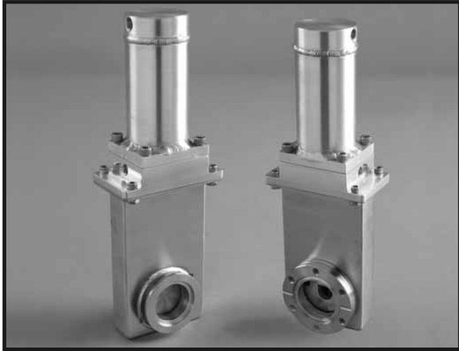
Valve on the left has NW-40 flange. Valve on the right has special 2.75 In. Conflat® flange. Standard practice is for bolt circle to straddle center line.
