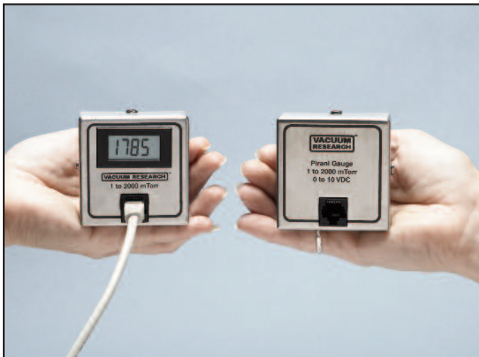
The instrument on the left shows the optional digital display. All models provide both 0 - 10 V and 4 - 20 mA linear outputs for your PLC.
