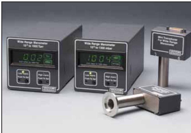
On left is an instrument calibrated in Torr and on the right an instrument calibrated in mbar. Transducers are available with all popular flange styles
